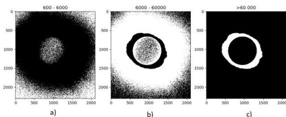
Fig. 3. The pixel distribution in the raw image, a) the pixel value level is in the range of 600 - 6000, b) pixels with a value of 6000 - 60,000 and c) pixels with a value higher than 60,000.
