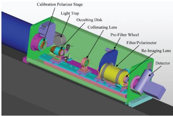
Fig. 2. Solid model rendering of the CoMP instrument package. Light enters through the blue tube on the left [12].
